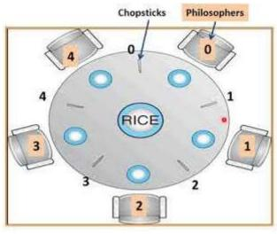
The design of the problem was to illustrate the challenges of avoiding deadlock, a deadlock state of a system is a state in which no progress of system is possible. Consider a proposal where each philosopher is instructed to behave as follows:
