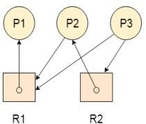
Using Resource Allocation Graph, it can be easily detected whether system is in a Deadlock state or not. The rules are
